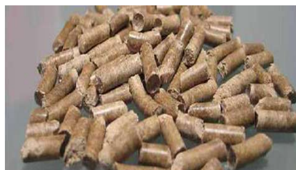
Figure 5 Pellets. Note: Pellets produced from rice husks. Fountain.: [25]
