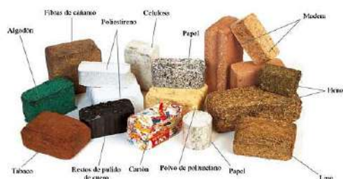
Figure 6 Briquettes. Note: Briquettes of different materials and shapes. Fountain.: [27]
