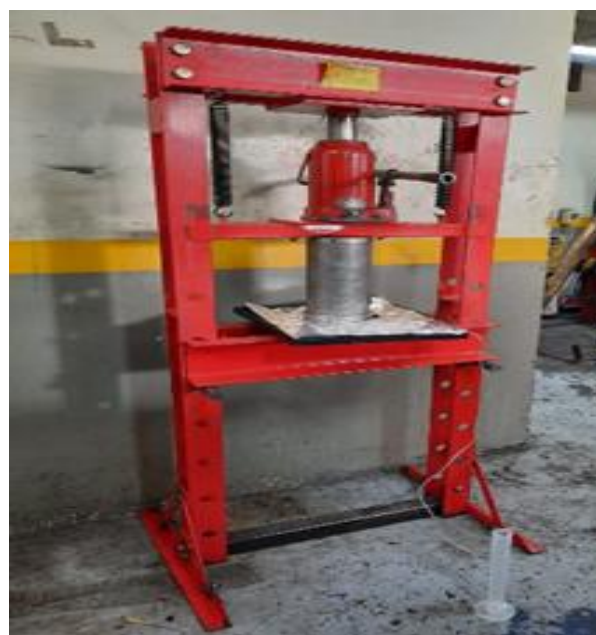
Fig 2. Hydraulic press with a capacity of 20 tons used for the pressing process
