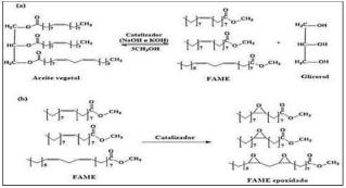
Figure 2. General reaction scheme for the process of obtaining epoxidized FAMEs (a) Transesterification of vegetable oils (b) Epoxidation. *Source*:[4]
