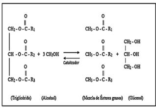
Figure 1. Typical transesterification of a triglyceride with methanol to produce fatty acid alkyl esters and glycerol. *Source:* [10]
