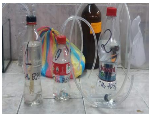
Percentage of CH 4 obtained from mixture I (0), mixture II (1) and mixture III (2).
