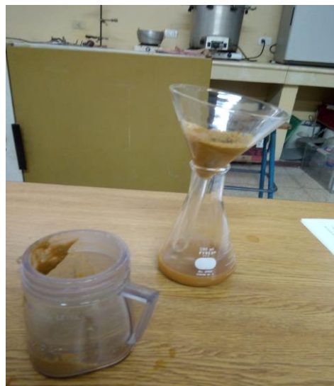
Fig. 8. Filtrate for Analyzing Titratable Acidity
