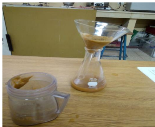
Fig. 6. Filtration of the Blend
