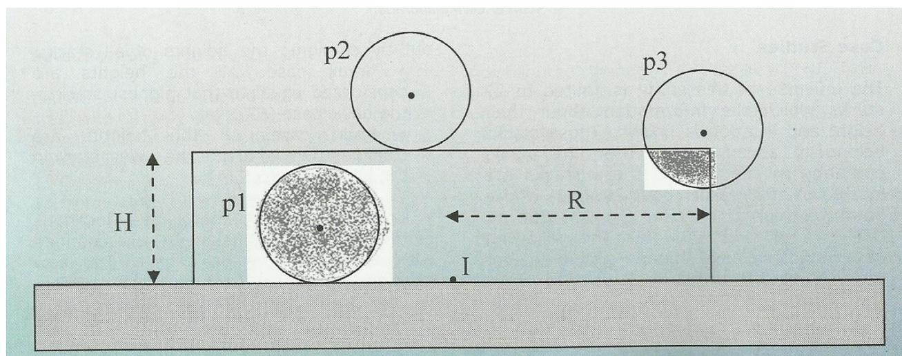
**Figure 4.** Schematic 2D view of the inmission volume considered for computing pollutant concentrations
