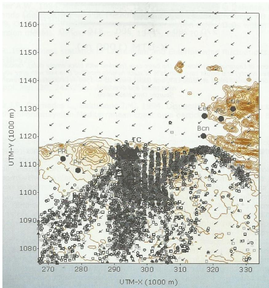
**Figure 5.** Location of Lagrangian particles for the basic case (marked with black empty dots), random case (marked with dark gray triangles empty) and height case with 25% of stack heights modified (marked with gray squares empty) for the XY plane, on the domain on February 11, 2006 at 18:00 LST, and surface winds (indicated by arrows that represent wind speed and direction). Locations of major cities are indicated by black filled dots and the stacks are indicated by black filled triangles.
