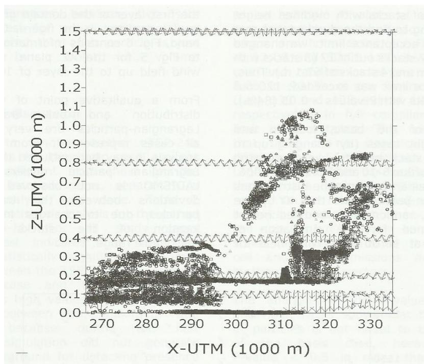
**Figure 6:** Location of Lagrangian particles for the basic case (marked with black empty dots), random case (marked with gray triangles empty) and height case with 25% of stack heights modified (marked with gray squares empty) for the XZ plane, on a domain zoom at 18:00 LST, and upper winds up to 1500 m (indicated by arrows that represent wind speed and direction).
