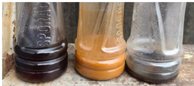
Figure 5. Liquid yield of PS, LPDE and PET respectively. Source: Own elaboration (2024).
