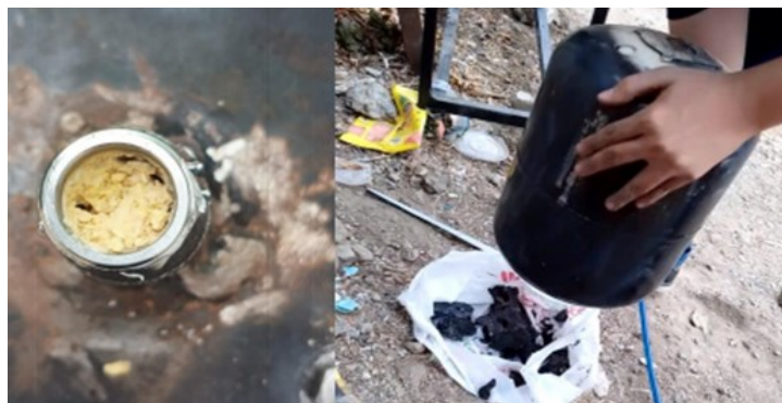
Figure 4. Material clogged in the pipes, Residue from the PET process. Source: Own elaboration (2024).
