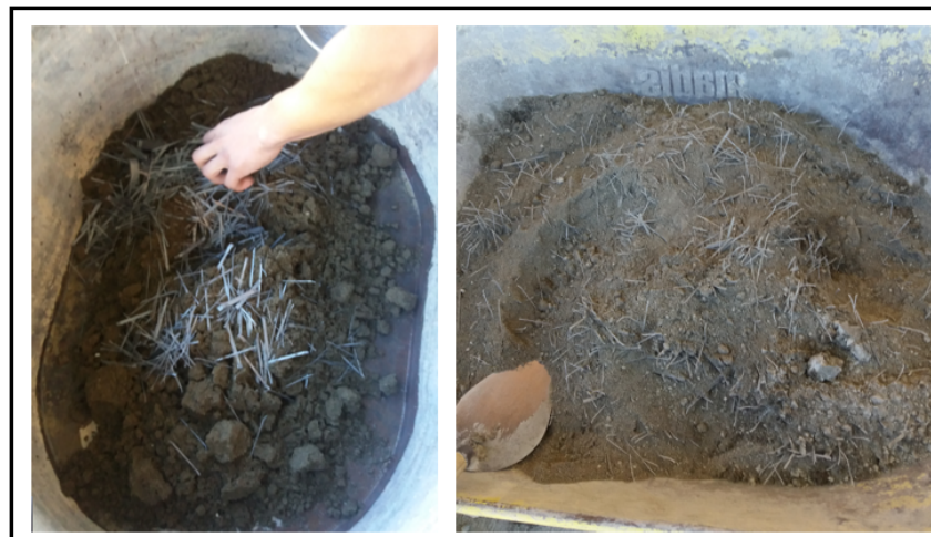
Figure 3. Manual mixing process of the mortar.
