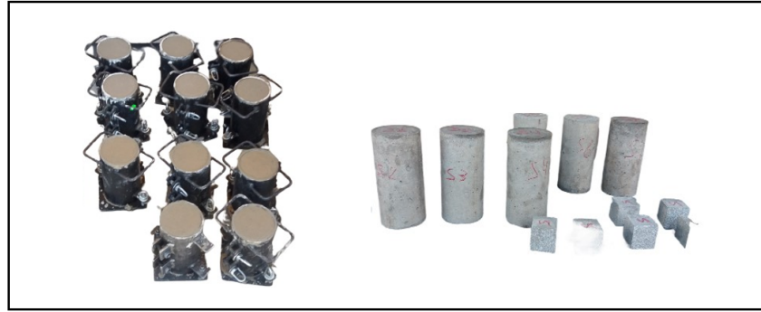
Figure 4. Casting and demolding of mortar specimens.
